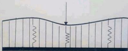
Fig. 10 Beam on elastic foundation analogy
